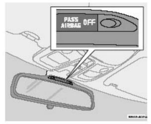
Occupant Weight Sensor (OWS) indicator light
